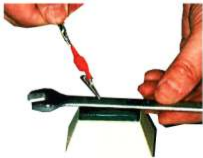
Deep etch marking in 15 seconds with adapter clip
