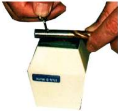
Etch round surfaces by rolling the item across the stencil
