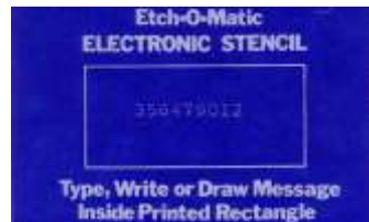
The special stencils can be used for 50 - 100 marks if handled carefully.
